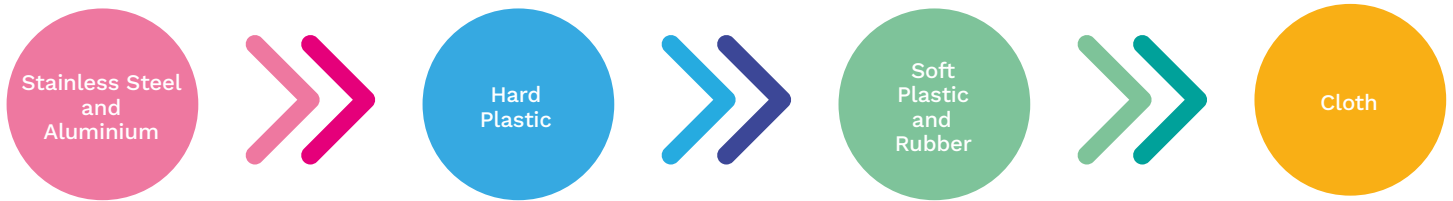
Figure 2: Diagram showing (from left to right) progression from materials that are typically easier to clean to those that are more difficult to clean.
