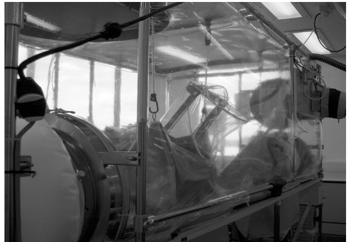
Figure 3: Soft-wall Sterility Testing Isolator (Image: Tim Sandle)
