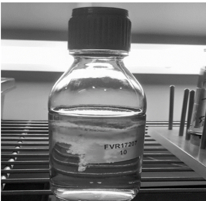
Figure 4: Sterility test bottle showing turbid growth (Image: Tim Sandle)
