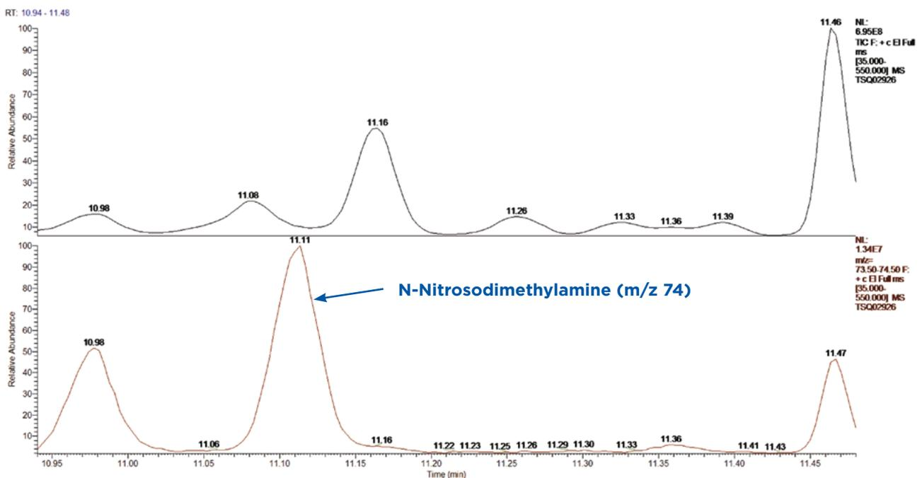
Figure 5: GCMS trace with extracted ion to show nitrosamine peak.
